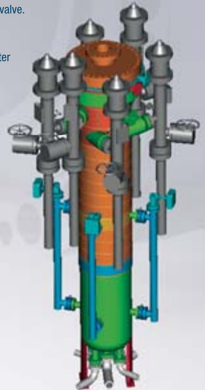
Figure 3 shows a Twister Hydrate Separator with six Twister tubes attached
