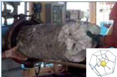
Figure 1 Hydrate Plug (insert shows methane hydrate)
