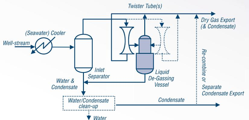
Figure 4 shows a typical Process Flow Diagram of a Hydrate Separator integrated within a Twister dewpointing system
