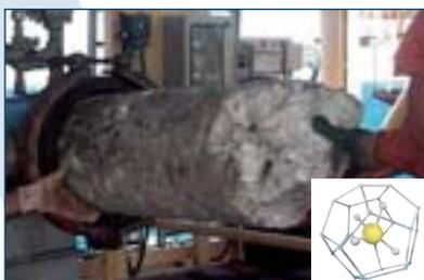
**Figure 1** Hydrate Plug (insert shows methane hydrate)
