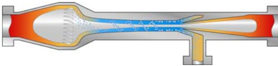
Figure 1: Artist impression of the “Twister Supersonic Separator”. The flow direction is from left to right. The separated liquid and slip gas are transported towards the bottom. The dry gas is continuing to the right.
