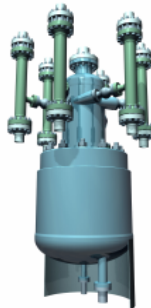
Figure 3 shows a typical Twister tube mounted on a vertical liquid degassing vessel.
