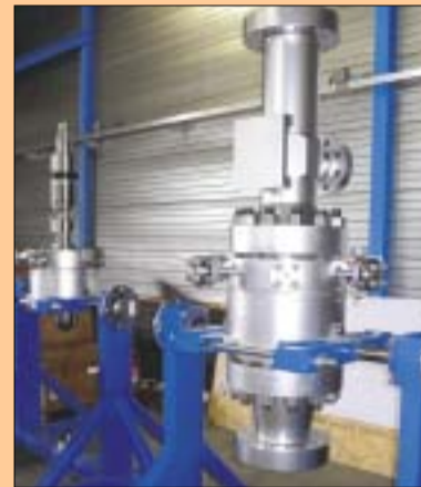
Fast mover: gas is rotated at supersonic speed in a Twister tube
